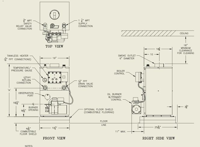
2. REFURN FITTINGS AND DRAIN VALVE SHIPPED LOOSE.
